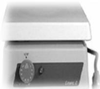
Water contaminated oil crackles when heated at 100° C, even in low concentration (0.1 %). The method consists in shedding a few drops of oil on a heating plate (100° C). Results are disclosed in %, between 0.1 % and 5%.
